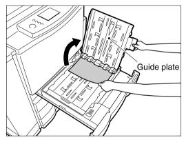
Push the lever, and then holding the handle of the lower guide plate, lift it slowly and fully.
